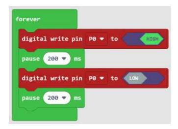
Load the program onto BrainPad Pulse and the RGB module should blink Red, awesome! Move the alligator clip from the Red pad to the Blue pad on the RGB module and the LED will now blink Blue.
