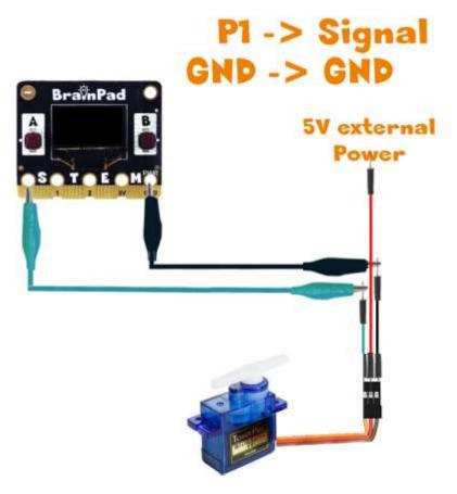
The "servo write" block is found under pins, under advanced. The block accepts 0 to 180 degrees, which is the angle of where the servo will be pointing.
