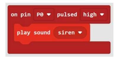
The event has the option to fire when the pin goes from low to high (pulse high) or from high to low (pulse low).
