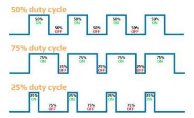
Controlling the level of energy on a pin (intensity on a light) is done by turning a pin on and off very rapidly. Now if we keep the duty cycle at 50% (that is half 1023), then the pin will generate a basic square wave. We then can change the PWM frequency to generate different tones.
