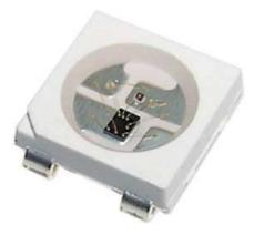
Those smart LEDs are chained and, therefore, they all can be controlled from a single pin on the controller. The "controller" in this case is BrainPad Pulse. The smart LED in the BrainClip kit is the LED Ring module.
