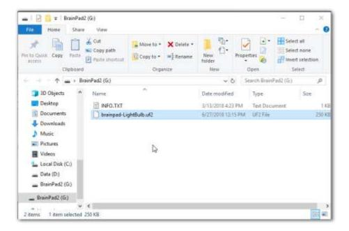
Once the file is done copying to the BrainPad Pulse, it will reset and execute the file you have just loaded. This will be our program from earlier that shows the light bulb on the screen "on start" and then blinks the LED "forever".
