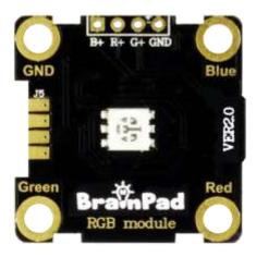
This is an RGB LED, meaning it has three mini light elements inside that are capable of producing Red, Green, and Blue colors. These are the primary colors used to make up any other colors. More on that in a minute.
