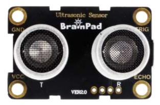
Sending a pulse starts with TRIG pin, the trigger. The response with the distance comes back on the ECHO pin. We will use TRIG on P0 and ECHO on pin P1.
